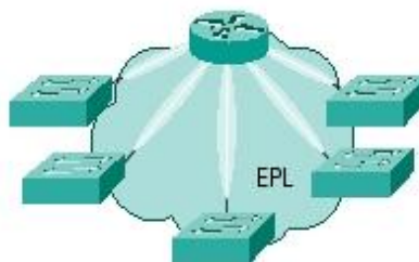
Figure 18 - Using Switches over EPL, Mapping Each Circuit to a Unique VLAN (Source: Cisco Systems, Inc.)
